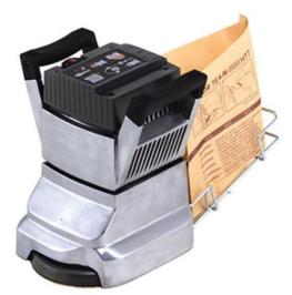
This edging floor sander is suitable for hard and soft wood floors, cork and composition floors and any solid wood surface that requires rapid sanding and levelling to a fine finish.
